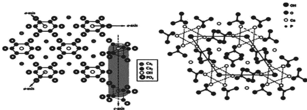
**Fig. 4:** Crystal structure of HAP exhibiting that the c-axis  $\perp$  to 3 a-axes lying at  $120^\circ$  of each other (left), and projection of structure of HAP on the 001 plane (right) [21].
