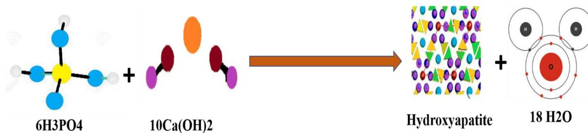
**Fig. 8:** Preparation of hydroxyapatite by the reaction of lime with orthophosphoric acid.
