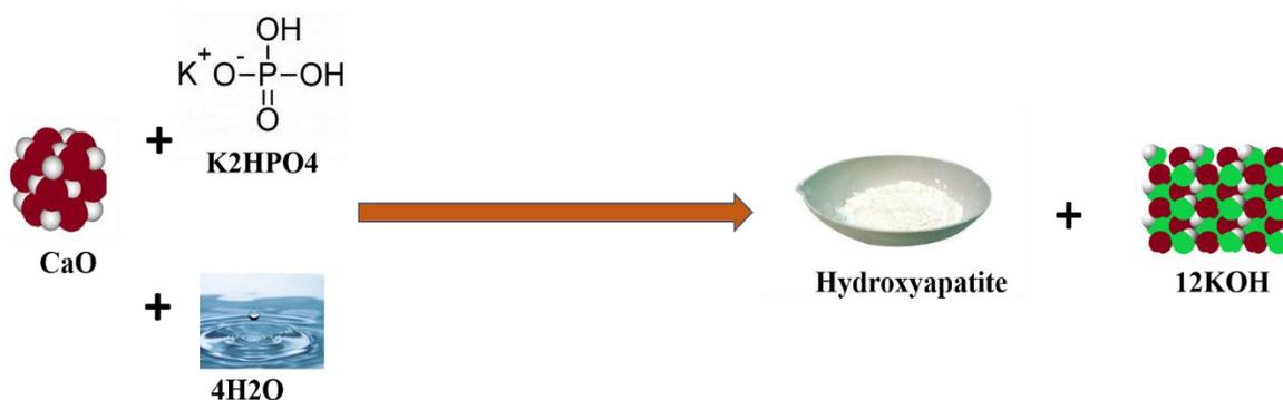
**Fig. 7:** Reaction of calcium oxide with dipotassium phosphate.
