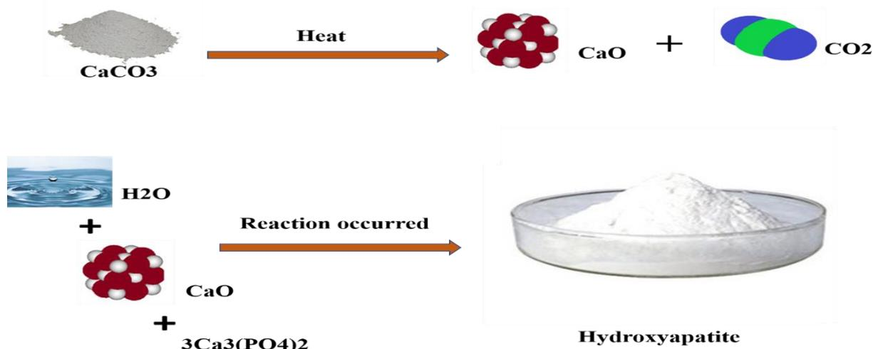
**Fig. 6:** Synthesis of hydroxyapatite by the reaction of calcium oxide with calcium phosphate in the presence of water.
