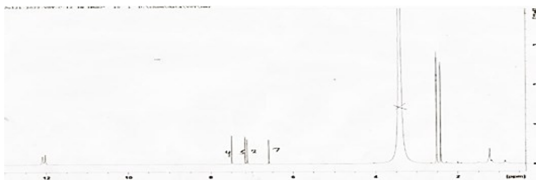
Fig. 2 ^1\text{H} -NMR spectrum for Emodin.
